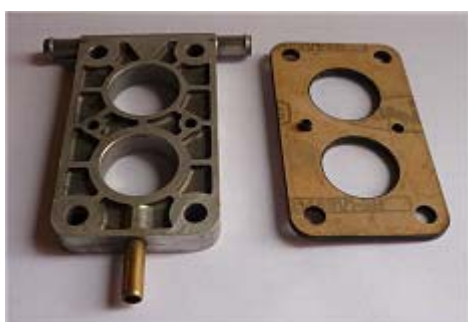
This picture shows the pre-heat flange and the upper insulating block.
