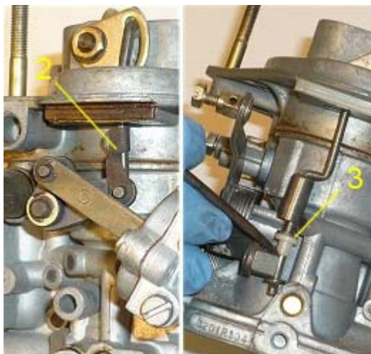
Remove the spring clip (2) from the choke pull off diaphragm linkage rod and detach the rod from the pivot lever.
