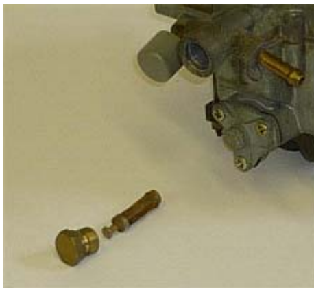
Remove the tubular fuel filter from behind the brass plug (14mm).
